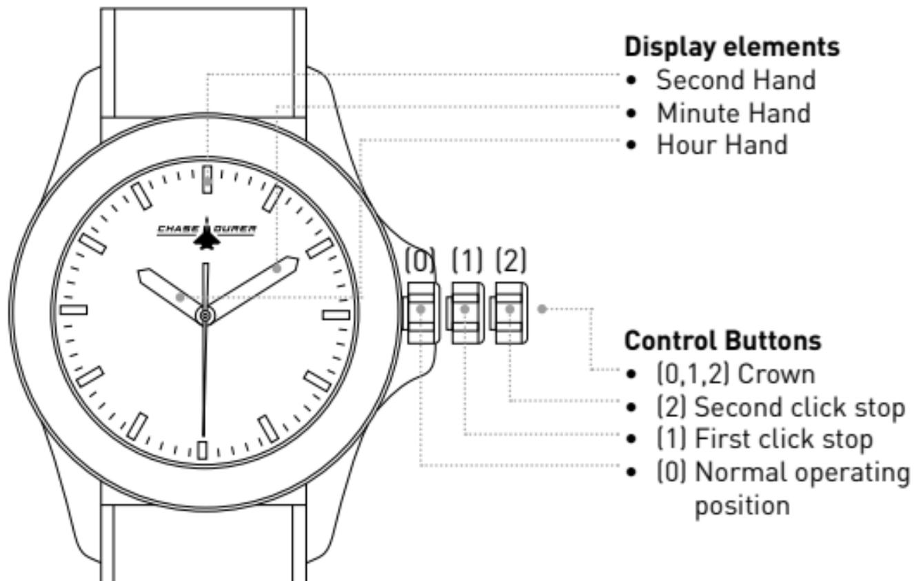
**Zero Position.** This is the position where the crown is at its innermost neutral spot. This is the secure position for normal operation of the watch.
