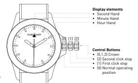
**Zero Position.** This is the position where the crown is at its innermost neutral spot. This is the secure position for normal operation of the watch.
